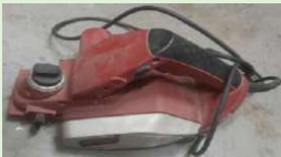
'SKIL' ELECTRIC HAND WOOD PLANNER (250V 50HZ 2.8A 650W)
